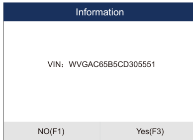
Figure 4-3 Sample Automatic VIN Reading Screen
